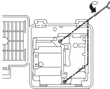
7. Grasp the bottom of the lamp as shown and pull it straight out.
